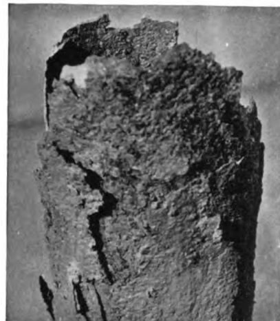
Fig. 65—Steel, Showing Aggravated but Typical Corrosion Resulting in Flaking or Scaling
