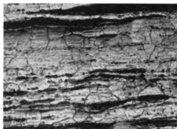
Figure 13—Micro section of wrought iron taken parallel to rolling. The black streaks are non-corrosive slag.
