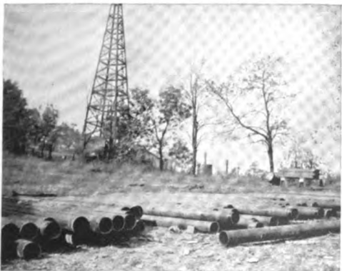
Byers genuine wrought iron casing, after eight years' exposure to the elements, on property of Donaldson Bros., Langloth, Pa. The pipe still looks like new and the threads are clean and perfect.
