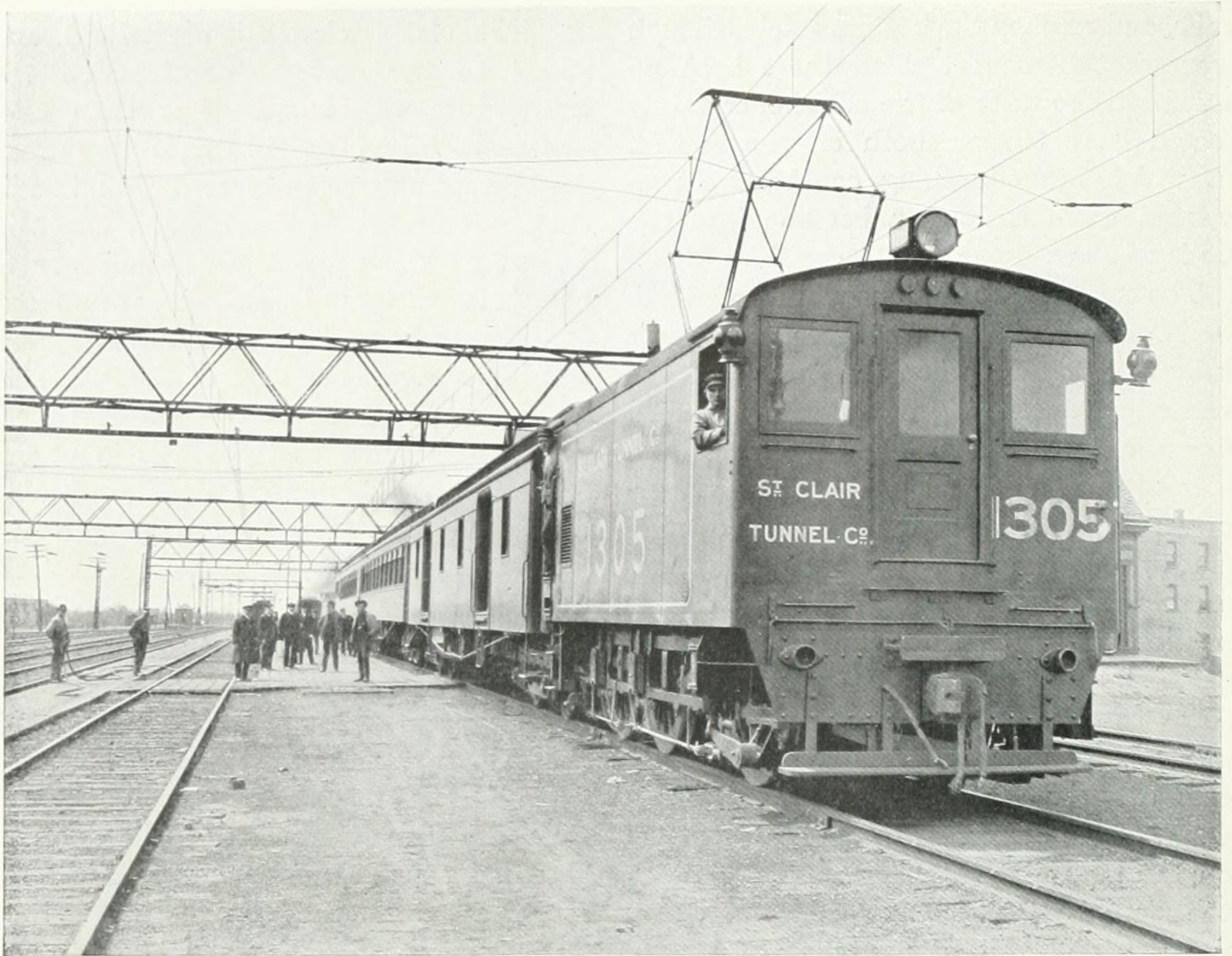
ONE OF THE ELECTRIC GIANTS WHICH "WORKS" THE ST. CLAIR TUNNEL These locomotives are of 2,000 horse-power, and weigh 135 tons
